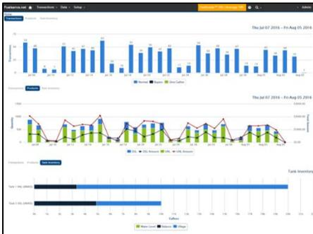
The Fuel Management System (FMS) collects data from each fuel transaction. It communicates via network cable or wireless connection to the cloud. This information is then accessed through the user's FuelServe.Net account on any device using their web browser.
